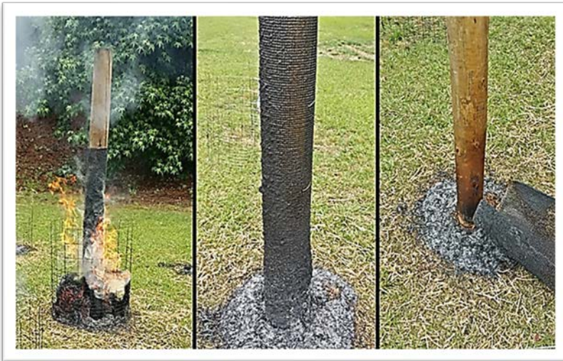
Figure 15. Fire resistant mesh wrap demonstration
